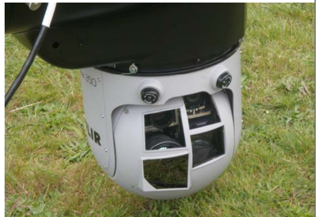
Figure 12: The Corona 350 Airborne Sensor Package
