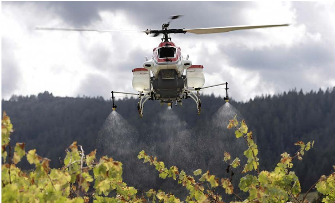
Figure 10: Yamaha R-Max Helicopter Spraying Vegetation
